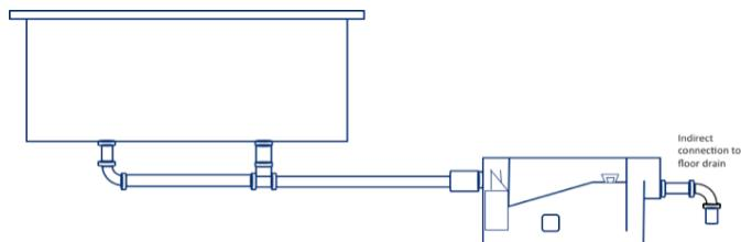
The Goslyn outlet may discharge either indirectly (e.g. into a floor sink as shown on the left) or directly to a drain pipe.
