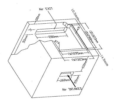
Table cut off size: 298 mm x 295mm Air In-Take Hole: 55(H) x 160 (W) mm Air Out-Take Hole: 55(H) x 160 (W) mm
