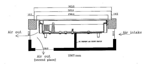
Remarks: Keep good air intake and outlet space is very important for good quality and function for this induction cooking device. Recommend to keep a open underneath the table not smaller than 200cm<sup>2</sup> (50x400mm) for fresh and cool air can be used for cooling the induction components (Air in-take hole, and air out-take hole).
