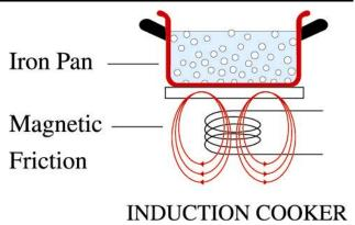
A high frequency (20-35KHz) induction coil underneath the surface ceramic top plate heats the cooking utensil by magnetic friction. The heat is produced directly within the pan. It is controlled by electronic circuit to offer superior performance and functions. During cooking, no energy is lost between the hob and the food. When you switch off, the cooking is stopped immediately.
