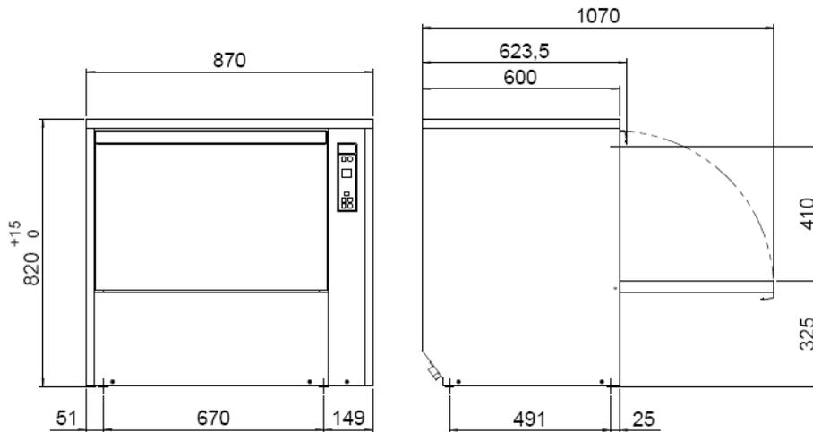
The machine height decreases by 4 mm when the feet are turned in completely.
