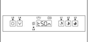
"on" = **the minimum temperature of rinse** as set, independently from the intake water temperature, the nominal duration of cycle may be extended by a few seconds.
