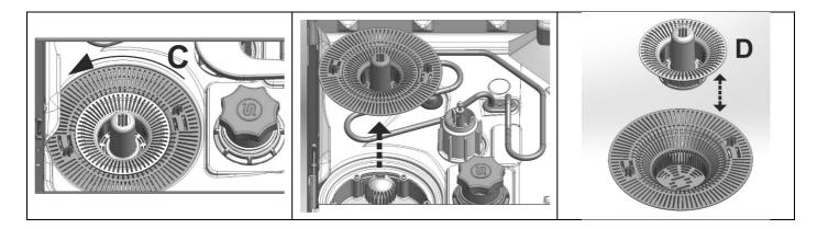
When removing the filters, do not let the coarse residues fall into the basin under the filters; clean and rinse them thoroughly, then re-insert them correctly; do not use sharp or pointed objects. If present, clean any limescale deposit to prevent accumulation;
