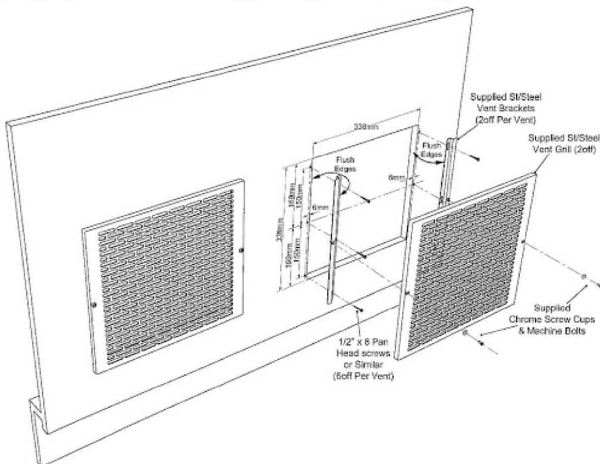
4. Drill a pilot hole & secure brackets using 1/2" (12mm) x 8 pan head screws or similar.
