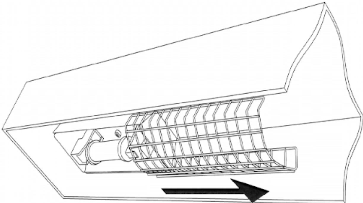
3. Remove faulty lamp by pushing to one side then pull down.
