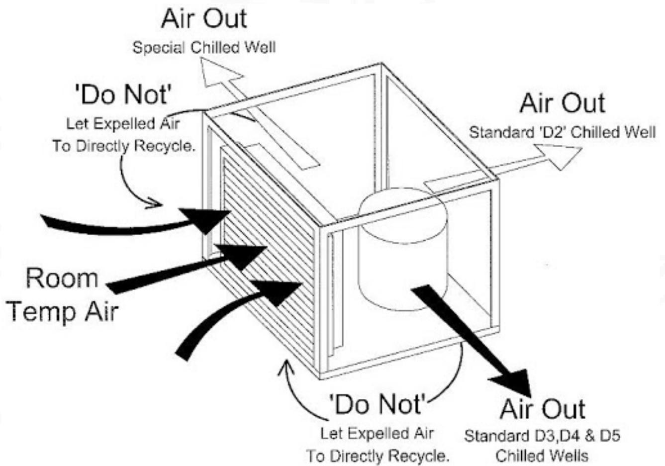
Where the drop-in requires boxing in the 'Plenum Duct' supplied should be fitted to fill in the void between the drop-in body & the shop-fitted counter panels.
