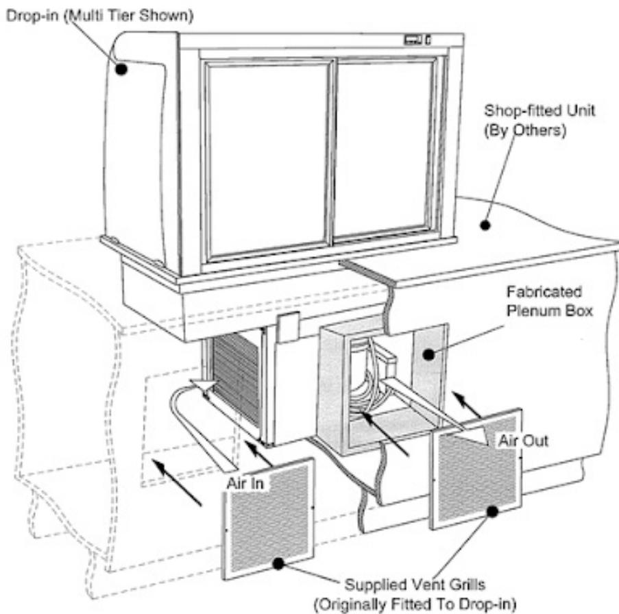
Plenum Duct in Situ, a 'plenum duct' will be required in certain situations to stop expelled air from the compressor being directly recycled into the coil vent. This box should be fitted to suit the gap between drop-in and the counter panel.
