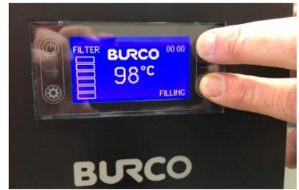
6. Press & hold the UP & DOWN buttons for 3 seconds to reset filter alarm on controller.
