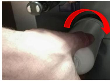
5. Twist new cartridge clockwise until locked in position
